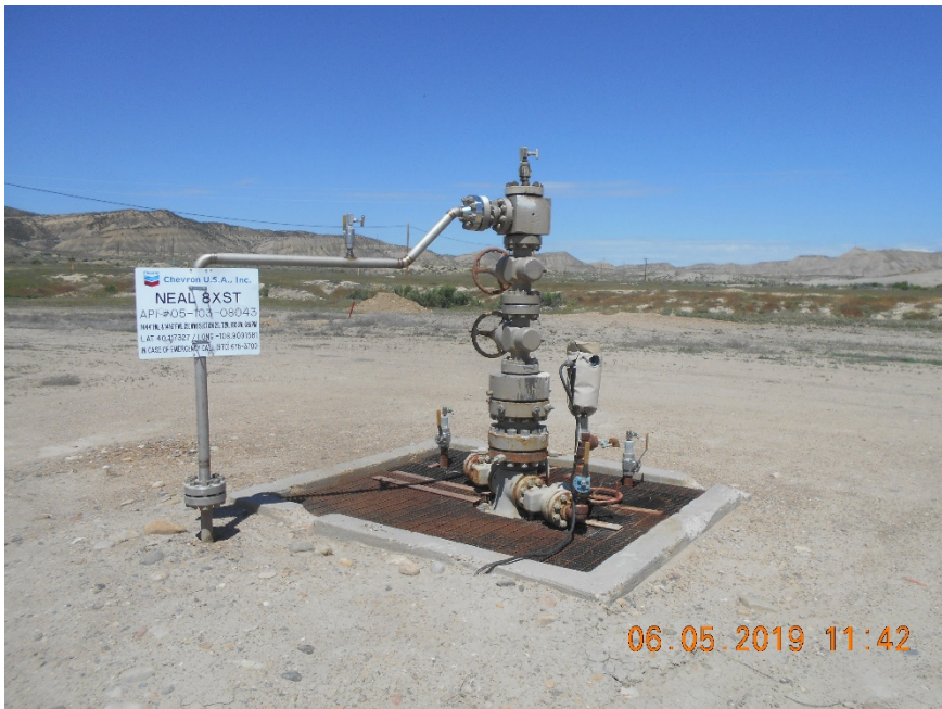
Injection wellhead
