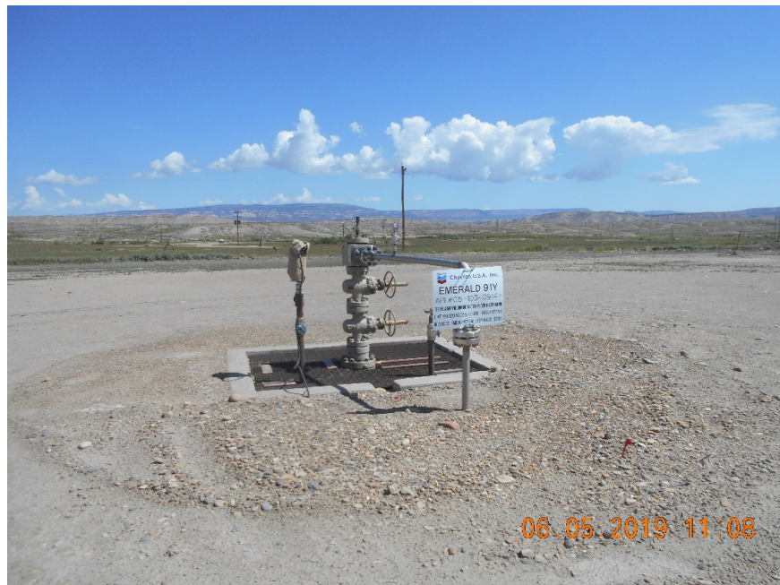
Injection wellhead
