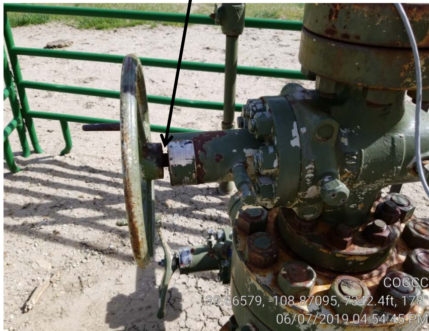
Photo 2. Wellhead valve gas leak.
