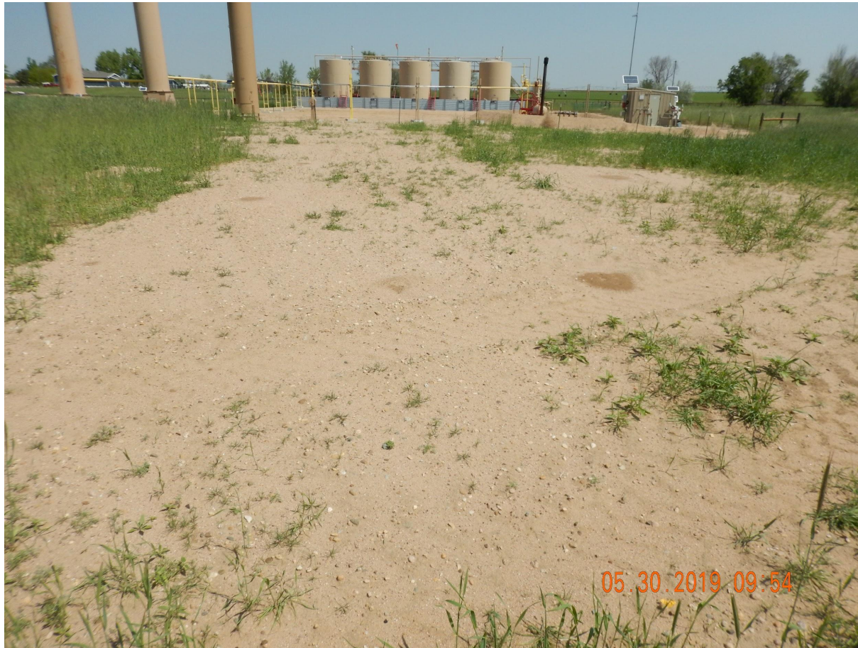
Photo 1. Photo taken from a portion of the flowline area, facing North. Photo illustrates a flowline area disturbance that has not been properly reclaimed per Reclamation rules. Photo illustrates bare ground with little, to no, establishment of reference area species.
