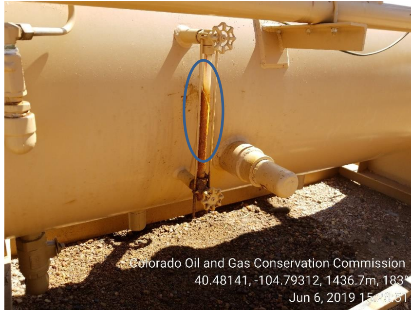
Photo 23: Cracked sight glass
