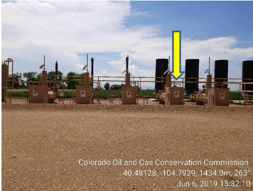
Photo 19: Separator with stained soil
