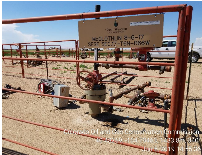
Photo 1: (TA) Wellhead; Unused equipment
