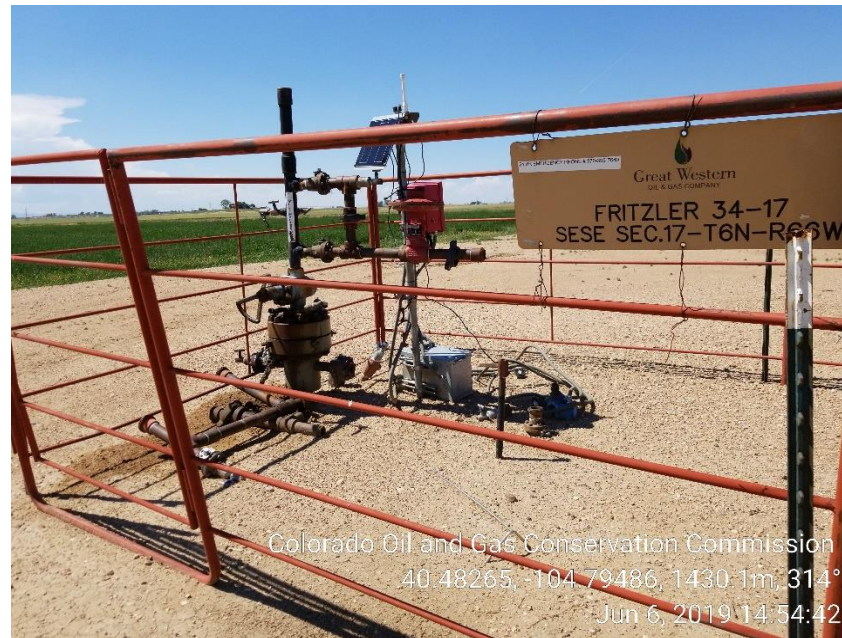
Photo 1: (TA) Wellhead; Unused equipment, Stained soil
