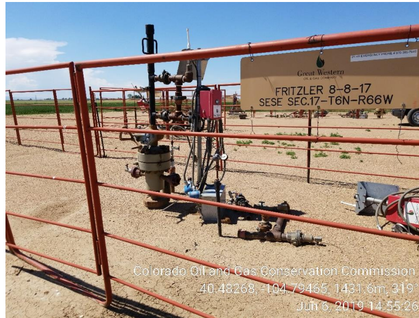
Photo 1: (TA) Wellhead; Unused equipment
