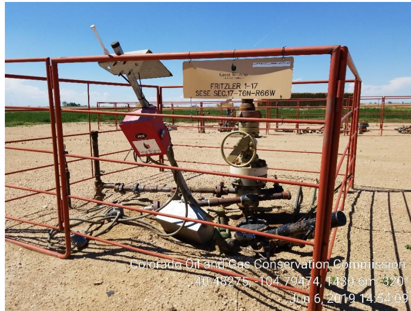
Photo 1: (TA) Wellhead; Unused equipment
