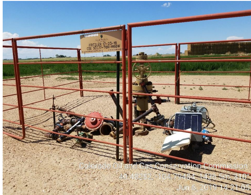
Photo 1: (TA) Wellhead; Unused equipment
