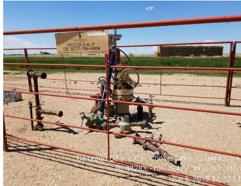
Photo 1: (TA) Wellhead; Unused equipment
