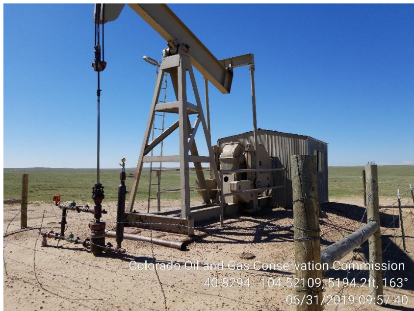
Photo 3 – Wellhead/Pumping Unit
