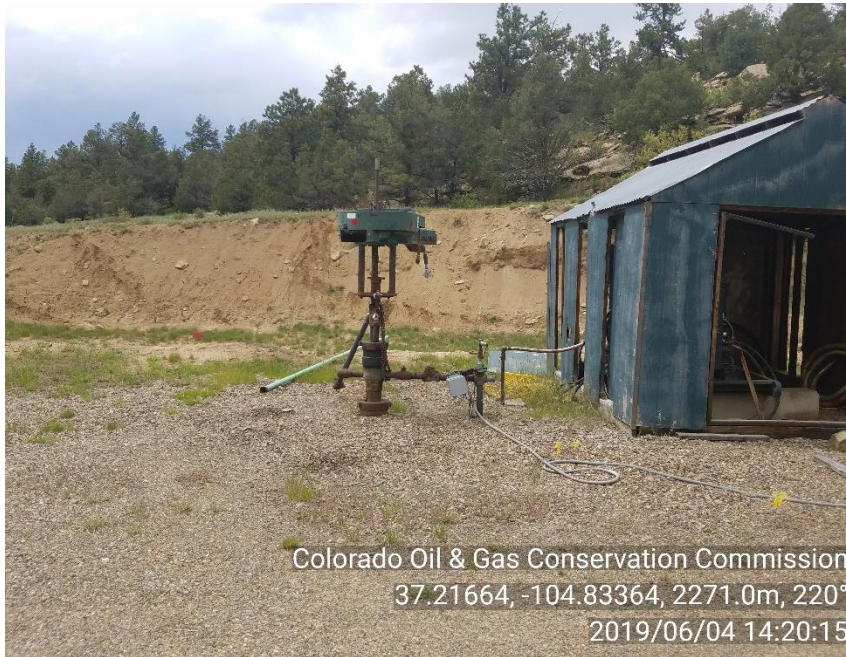
PHOTO 1: ORIGINAL WELLHEAD
