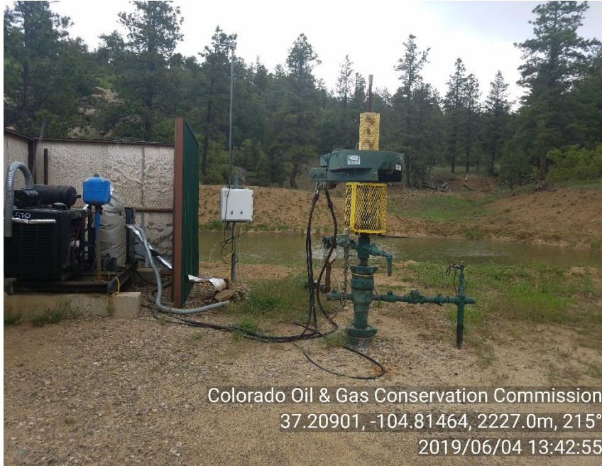
PHOTO 1: V WELLHEAD
