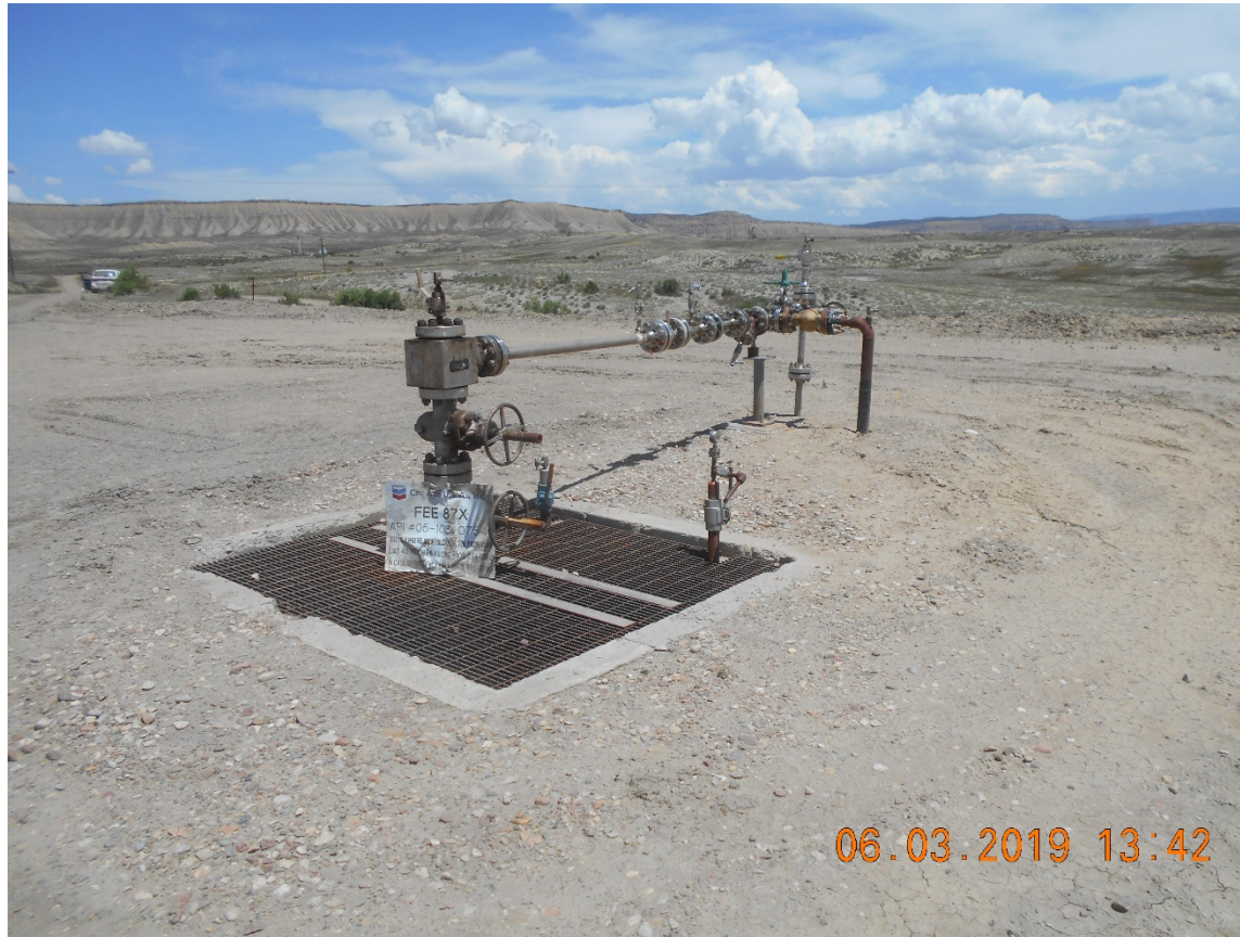
Injection wellhead
