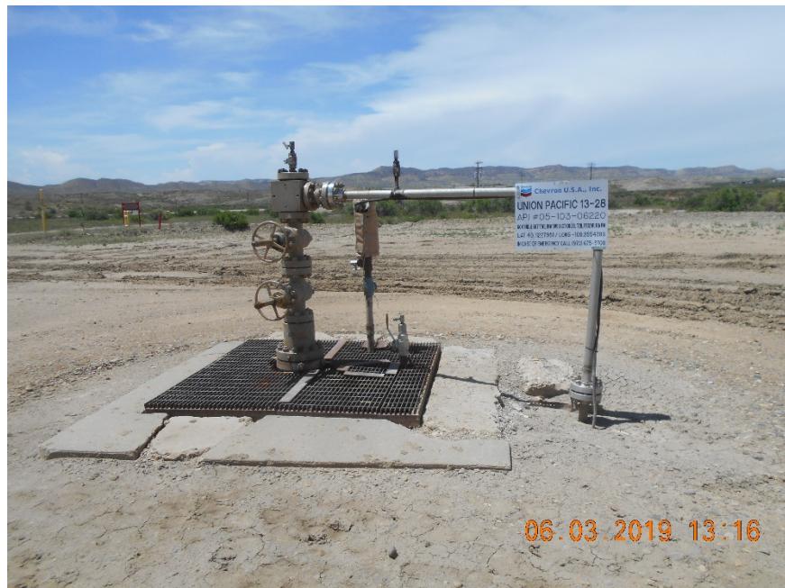
Injection wellhead
