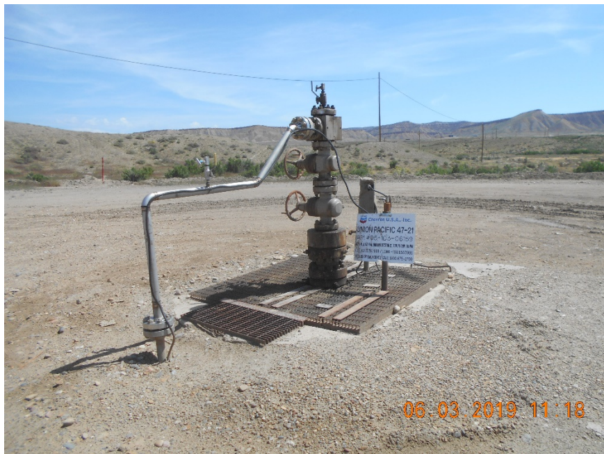
Injection wellhead
