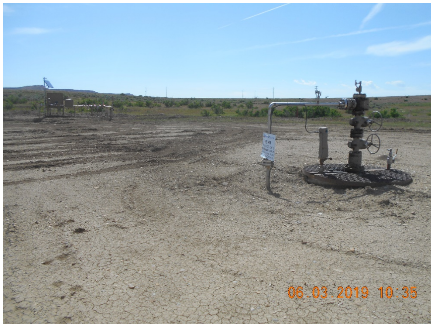
Injection wellhead
