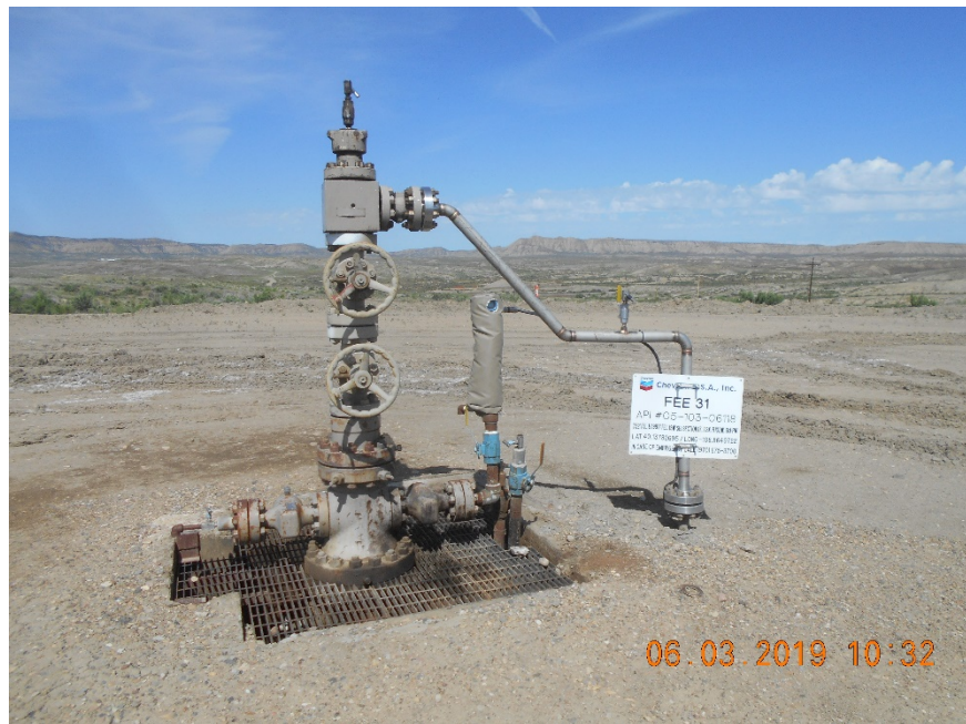
Injection wellhead
