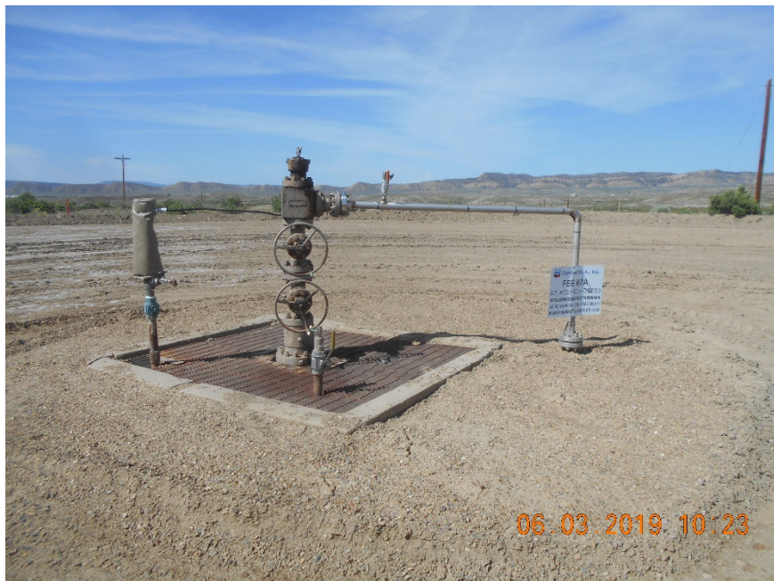
Injection wellhead
