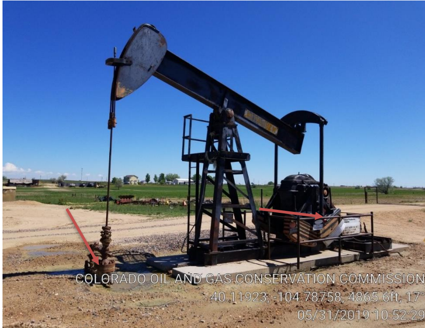
Pic 1 no cap on casing valve sign faded
