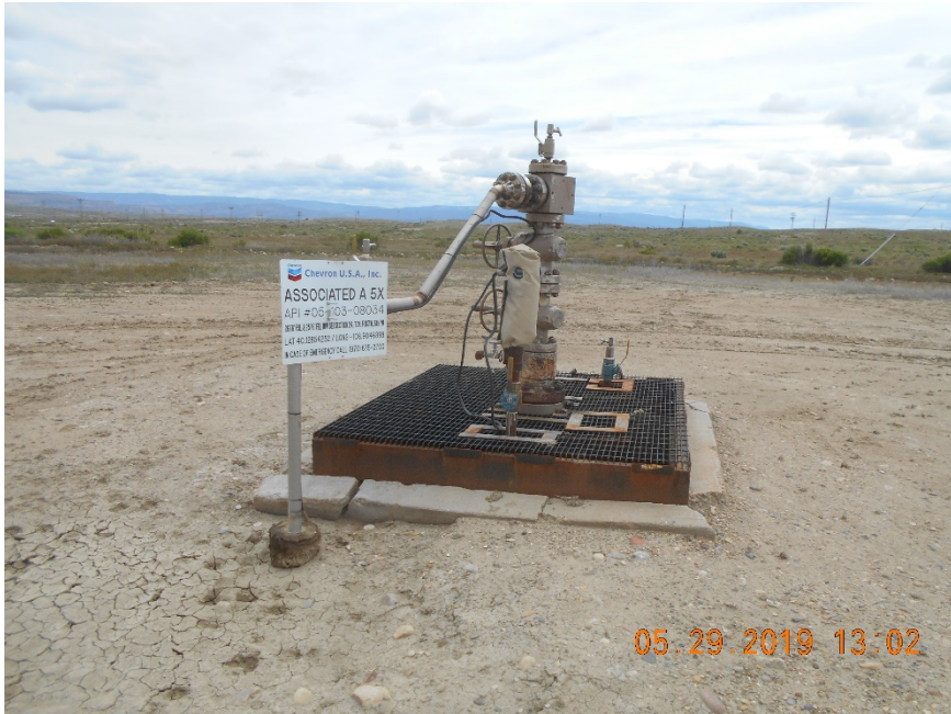
Injection wellhead
