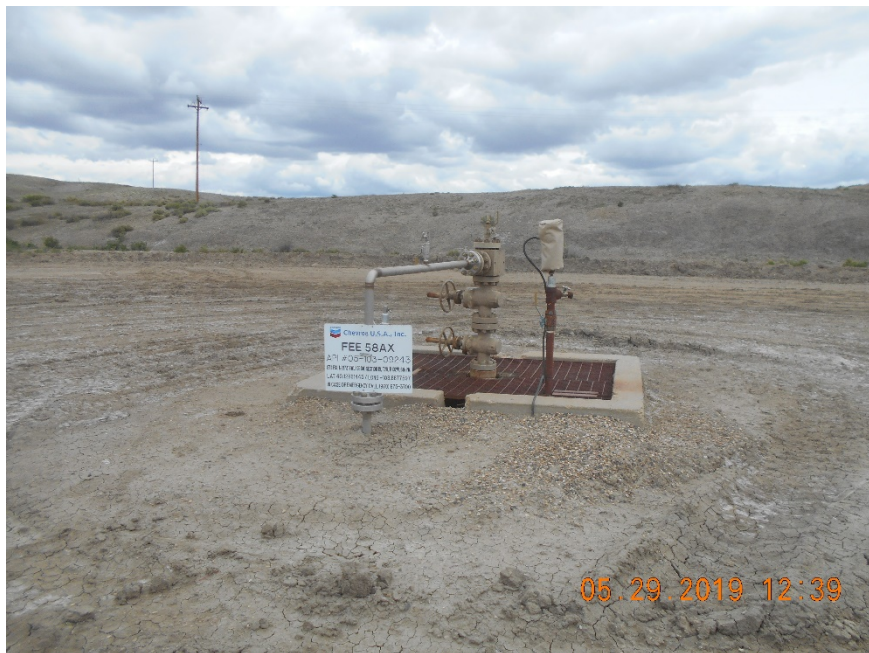
Injection wellhead
