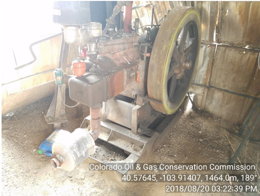
Photo #9 Nickerson 4 - Engine House Stained soil around engine base from prior insp.
