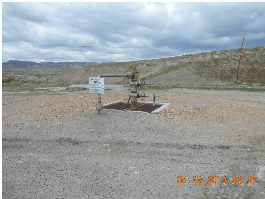
Injection wellhead
