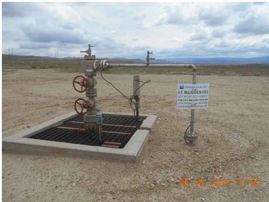
Injection wellhead
