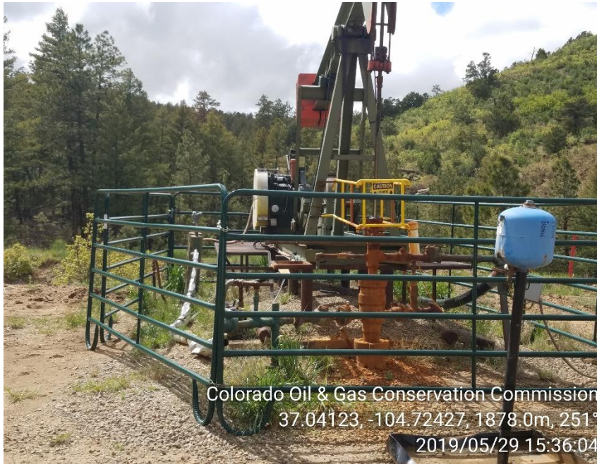
PHOTO 1: WELLHEAD/ IMPACTED SOIL AROUND WELLHEAD. Remove and dispose impacted material in approved manner, service and maintain equipment and self inspect to prevent recurrence of conditions per 1002.f(2) and 907" CA DATE 6/29/19
