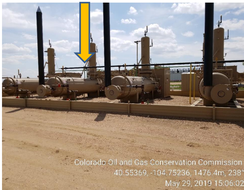
Photo 3: Separator with tubing inside housing.
