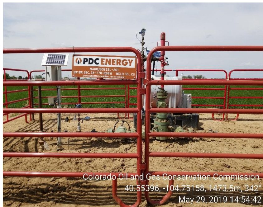
Photo 1: Wellhead w/methanol pump
