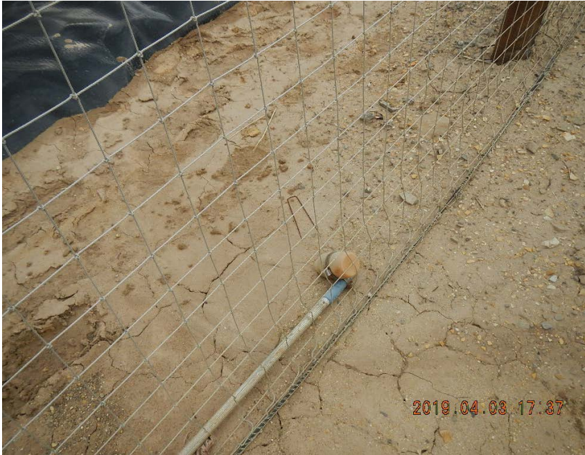
Sampler and wire anchor pin inside of pit complex.
