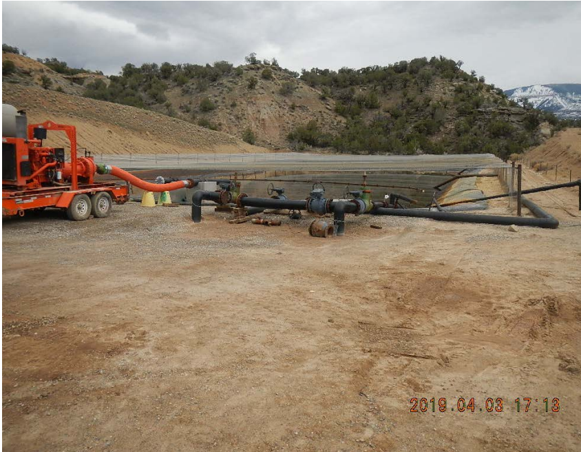
Manifold system cribbed with wood blocks, unused equipment, flow line directly on pit liner
