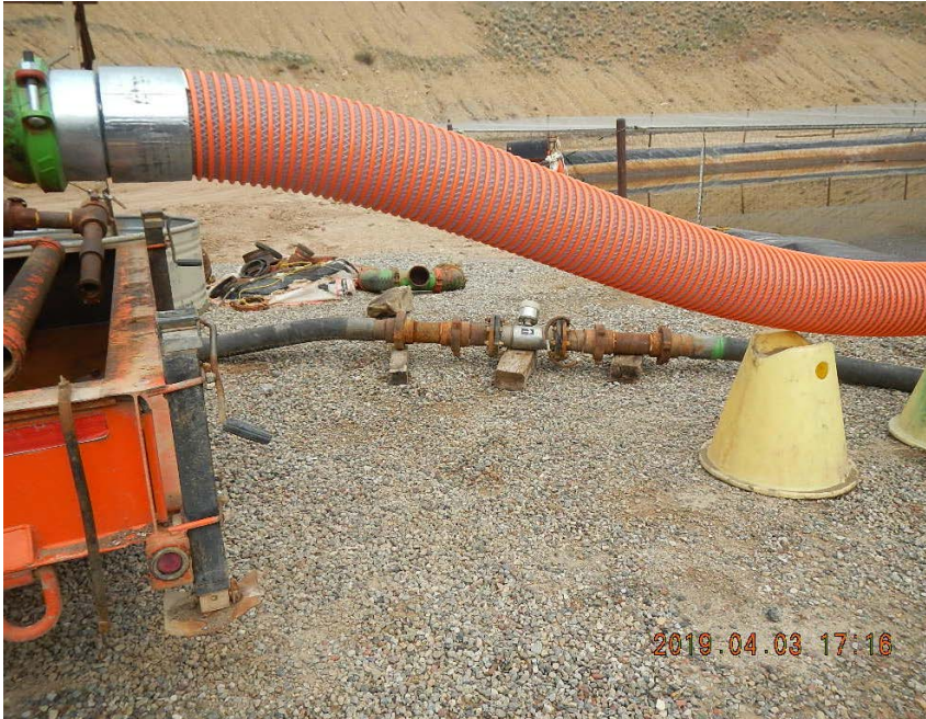
Unused equipment. Flow meter supported by wood blocks.
