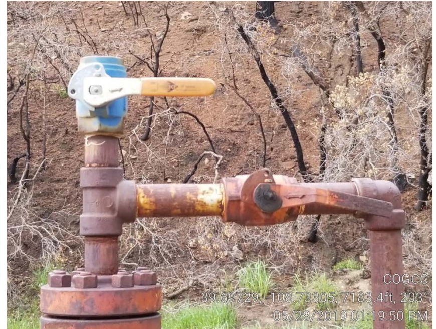
Photo 3. Well head leaking gas to the atmosphere.
