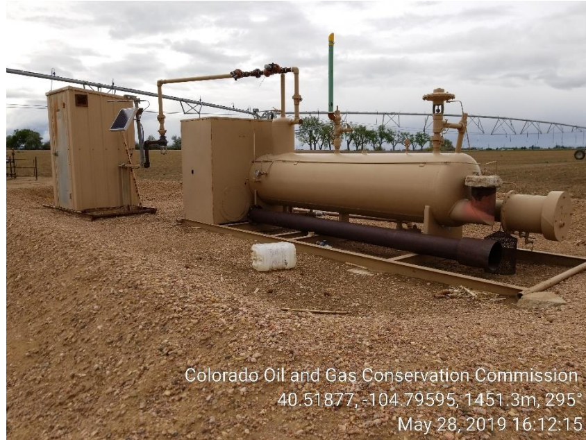
Photo 3: Disconnected separator.
