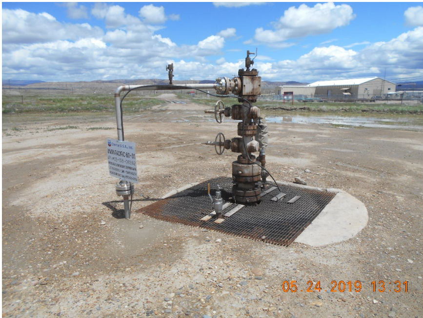
Injection wellhead
