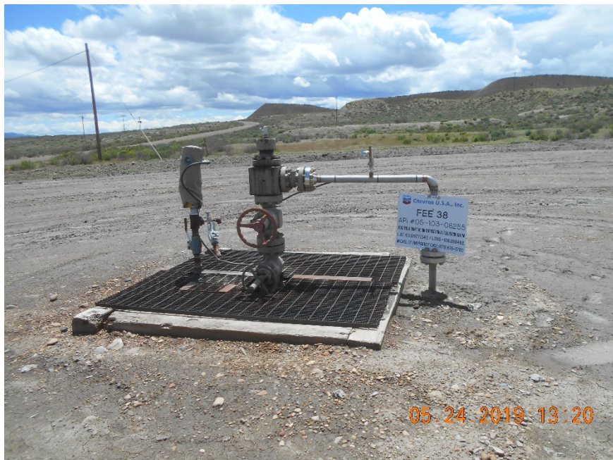
Injection wellhead
