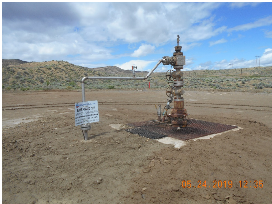
Injection wellhead
