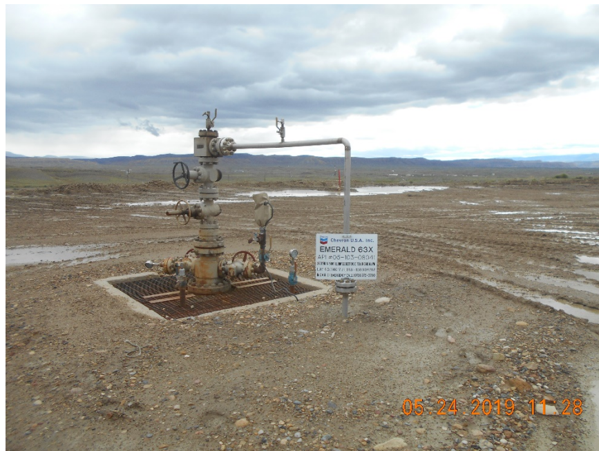
Injection wellhead
