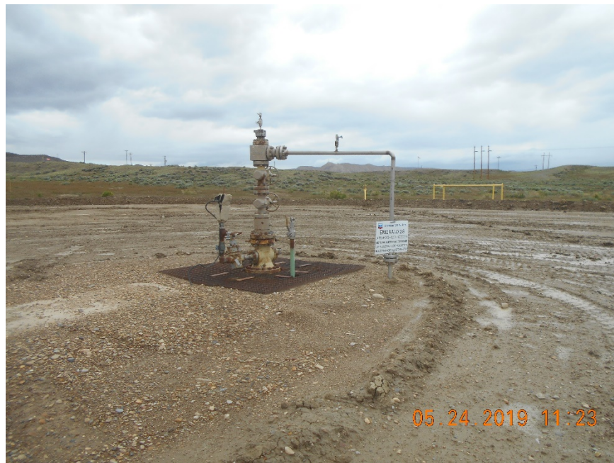
Injection wellhead
