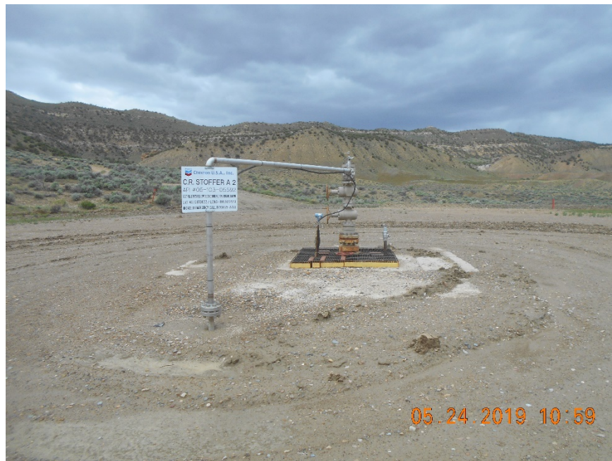
Injection wellhead
