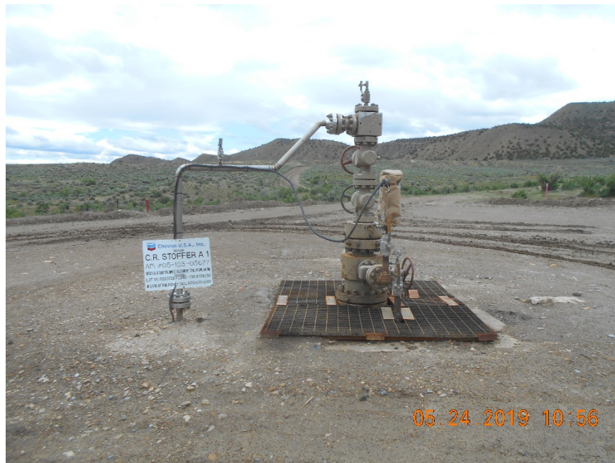
Injection wellhead
