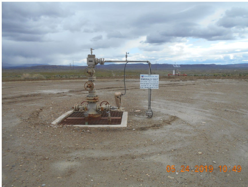
Injection wellhead
