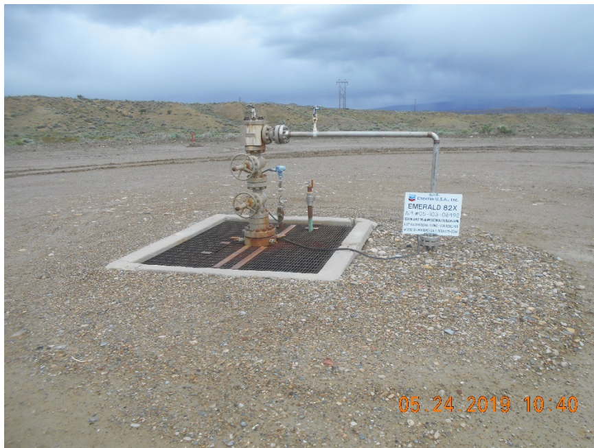
Injection wellhead
