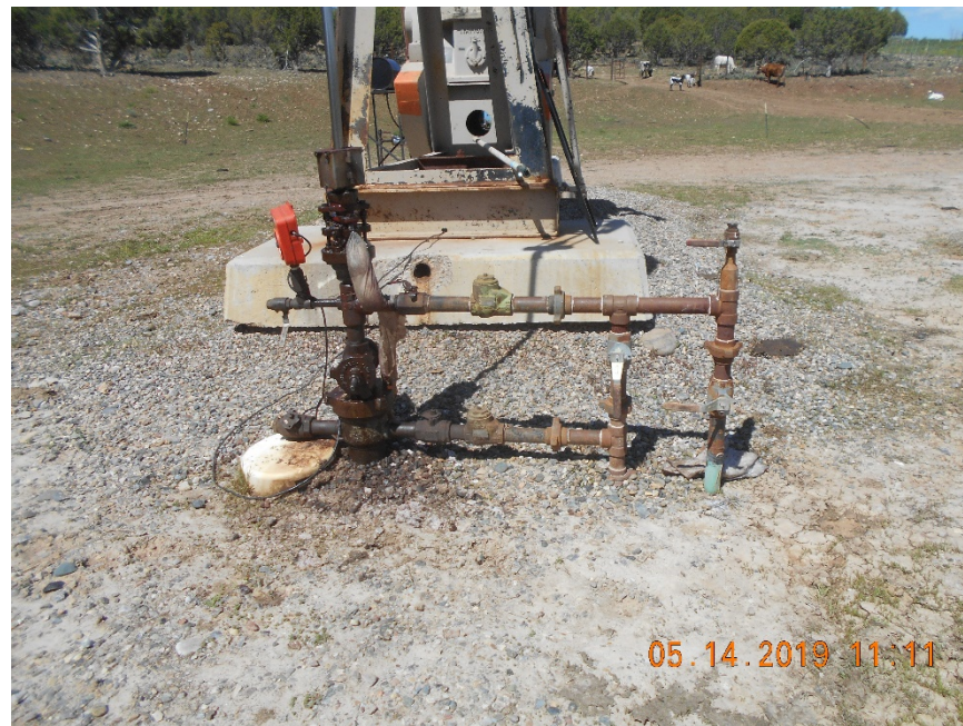
API # 05-067-09621 ARTFGANCE 33-7-14 #2A Wellhead with stained soil
