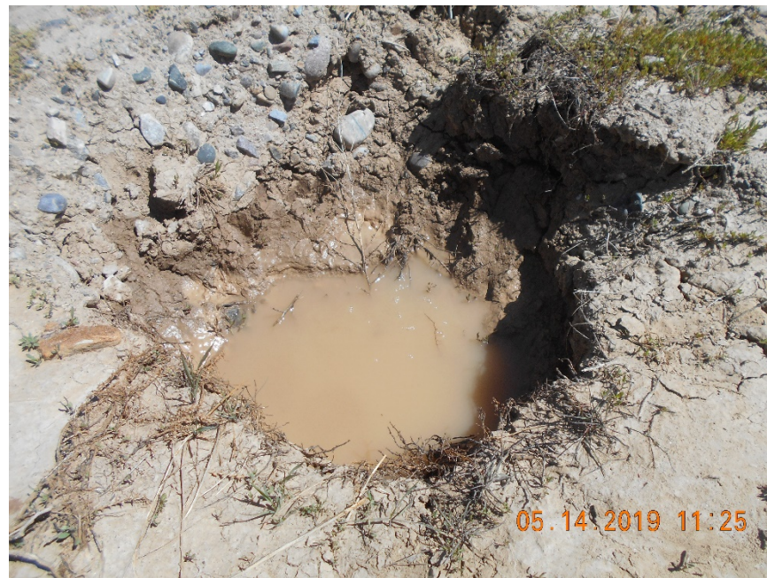
API # 05-067-09621 ARTFGANCE 33-7-14 #2A Washed out 10" diameter hole ~20' NE of wellhead. Noted changing fluid levels and intermittent bubbles.
