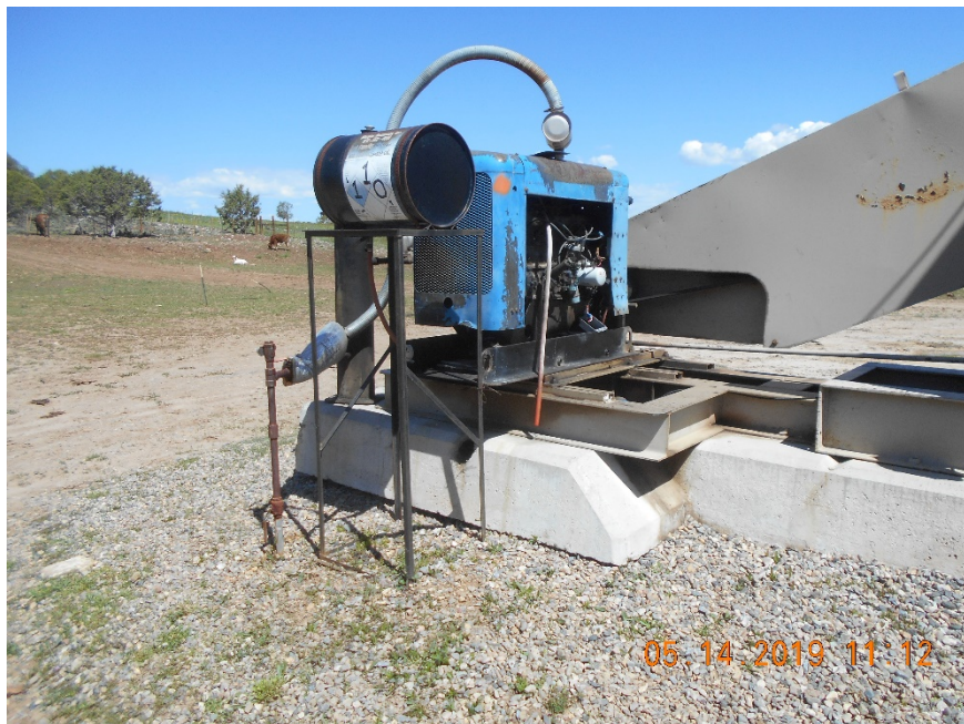
API # 05-067-09621 ARTFGANCE 33-7-14 #2A Motor oil container with no secondary containment
