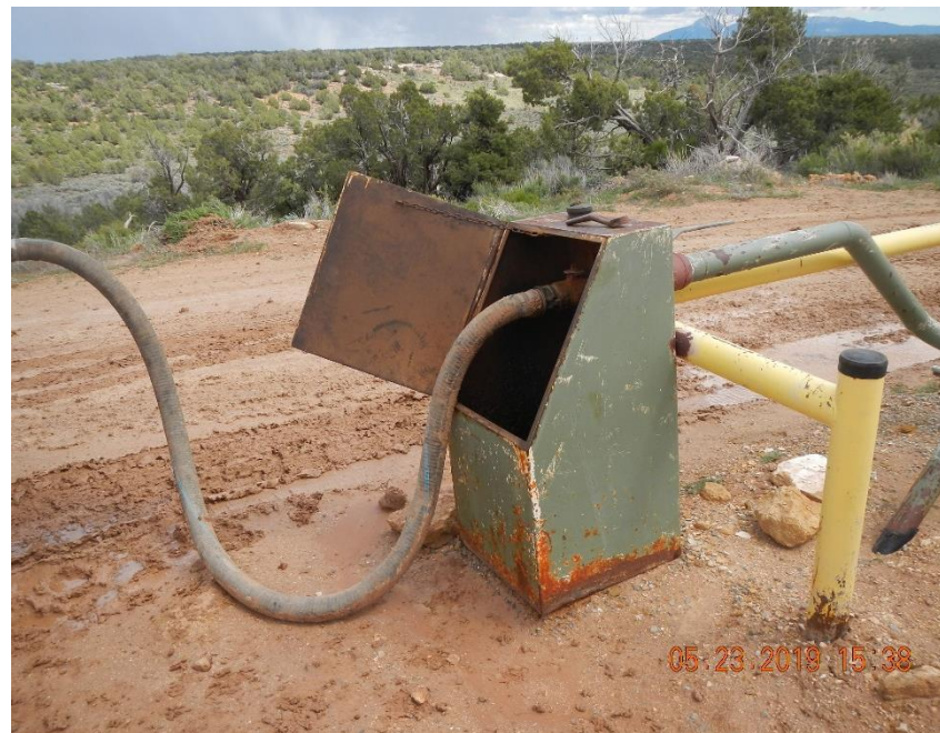
Drip pot at truck load out.
