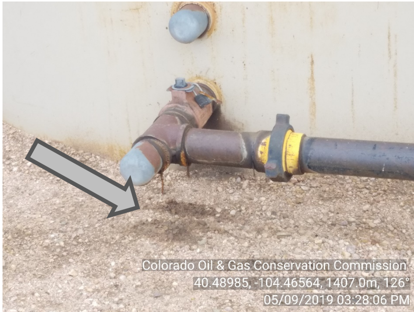
Photo #5 Peppler 17-12, 17-22 Battery East condensate tank - loadout Stained soil from prior insp.
