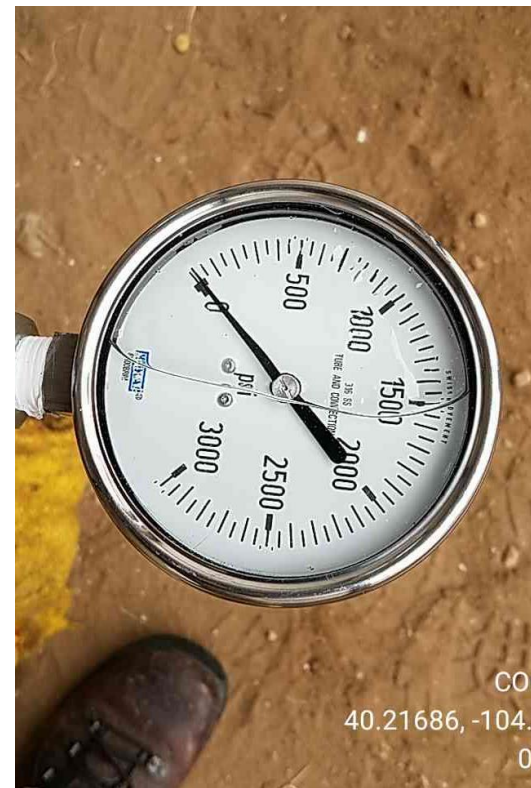
Photo 3 Initial Casing Pressure Gauge
