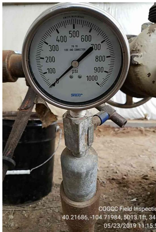
Photo 2 Initial Bradenhead Pressure Gauge
