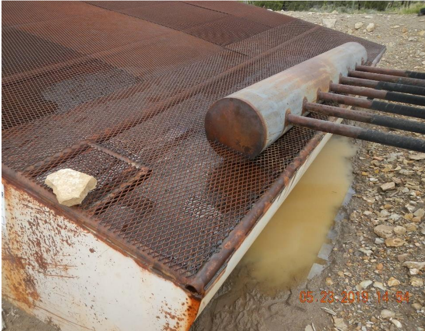
Contents of open topped vessel are overflowing.
