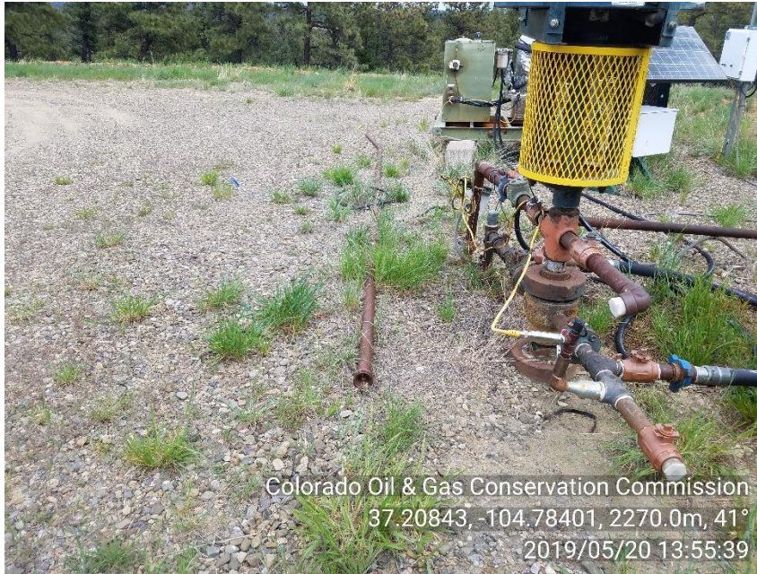
PHOTO 3: UNUSED EQUIPMENT (1 JT OF 2" PIPE LYING NEXT TO WELLHEAD. COMPLY WITH RULE 603.f. CA DATE 6/20/19
