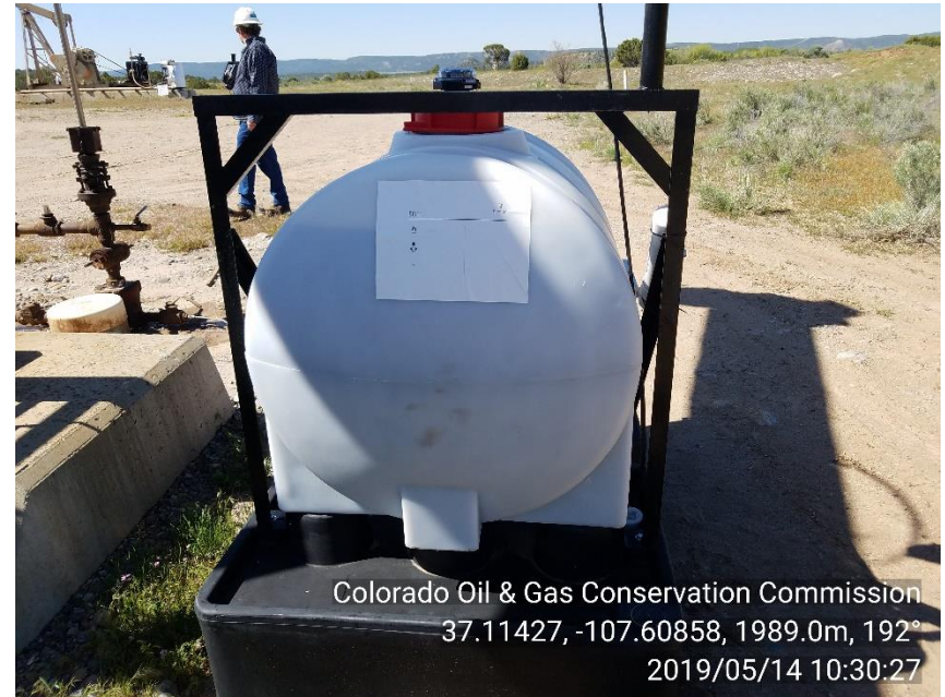
PHOTO 10: LABEL ON CHEM. CONTAINER NEAR WELL 33-7-9 #1 IS FADED AND NOT LEGIBLE. COMPLY WITH RULE 210. CA DATE 6/21/19
