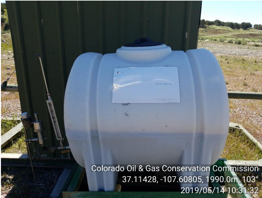
PHOTO 11: LABEL ON CHEM. CONTAINER NEAR METER HOUSE ON NORTHEAST EDGE OF LOCATION IS FADED AND NOT LEGIBLE. COMPLY WITH RULE 210. CA DATE 6/21/19
