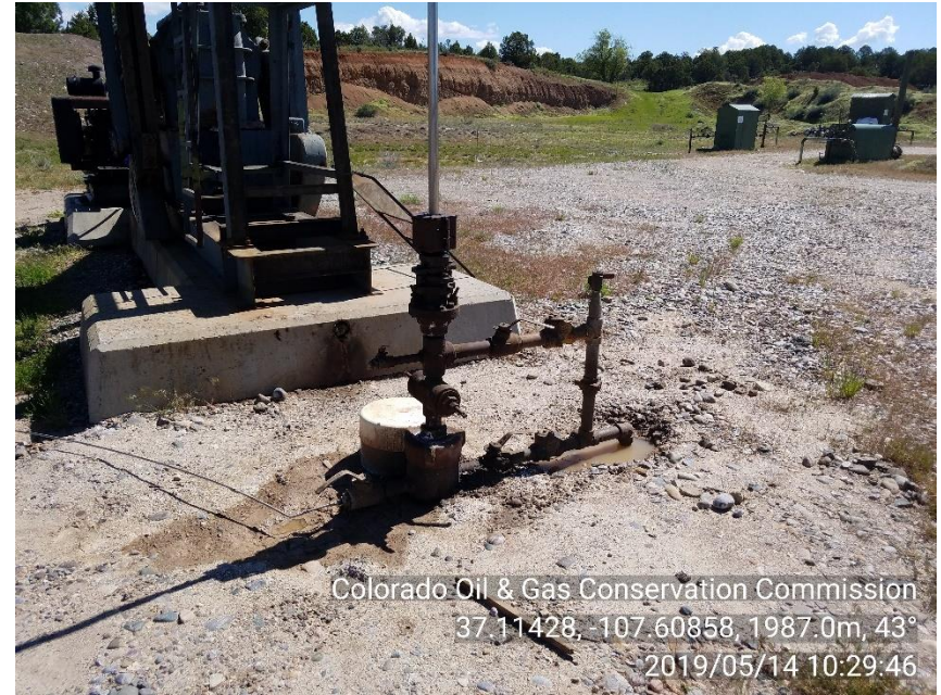
PHOTO 8: IMPACTED SOIL AROUND EAST OF THE 33-7-9 #3B WELLHEAD. Remove and dispose impacted material in approved manner, service and maintain equipment and self inspect to prevent recurrence of conditions per 1002.f(2), 907 & 906" CA DATE 6/21/19
