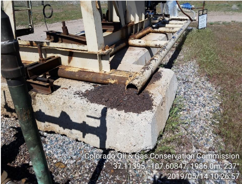
PHOTO 7: APPEARS TO BE RUST OR SCALE PILED NEXT TO PUMPJACK SKID ON THE 33-7-9 #3B WELL. REMOVE TRASH TO COMPLY WITH 603.f. CA DATE 6/21/19
