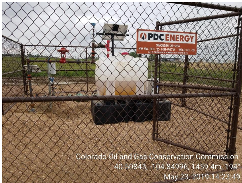
Photo 1: Wellhead w/methanol pump
