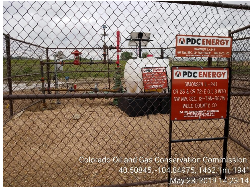
Photo 1: Wellhead w/methanol pump
